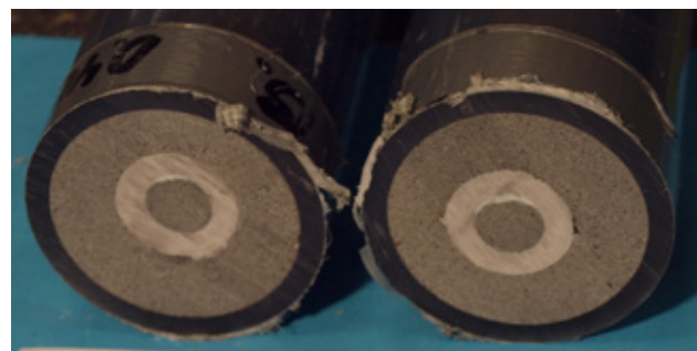
PC-Bolt M27/15 cut 500mm from each end.
