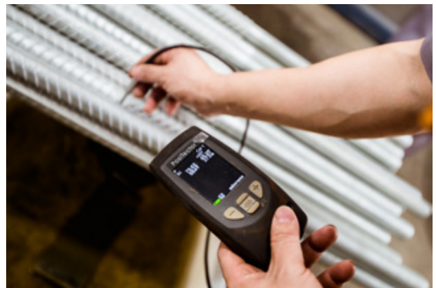
Control of coating thickness
