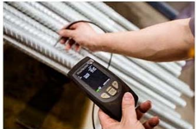
Control of coating thickness
